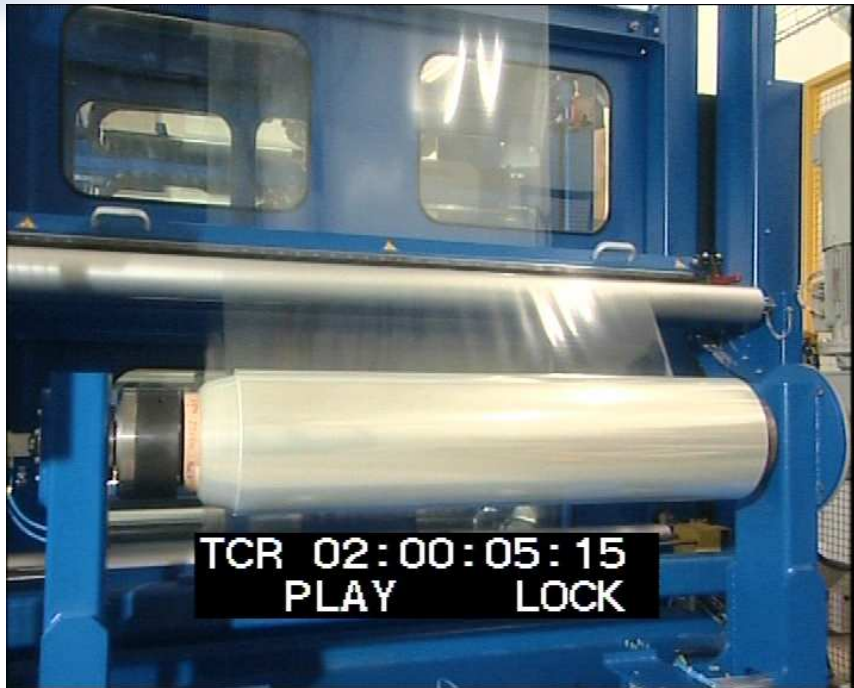
Inlet with the roll of polymeric film
